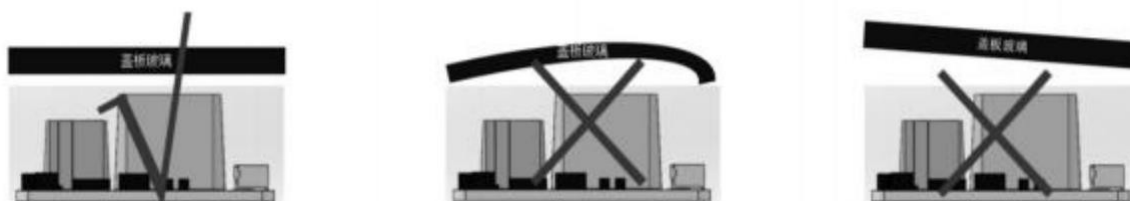
Figure 4 Installation diagram of shading film
